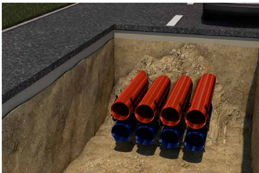
Minimum routing depth of cable ducts for heavy load traffic with SLW60 trucks
